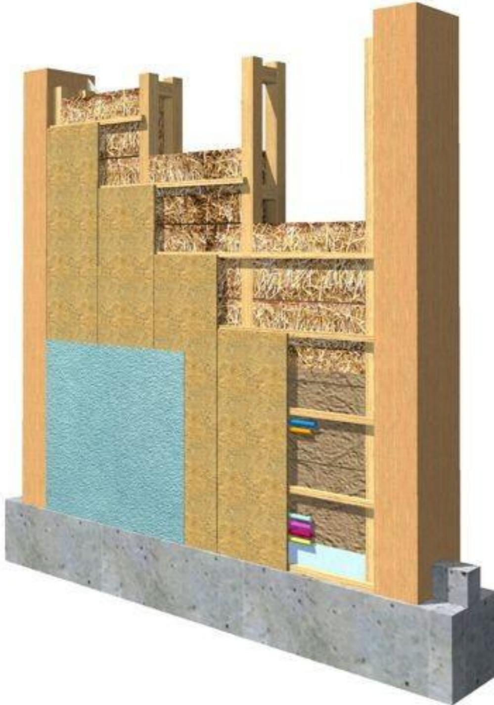
As is customary with all our infrastructure, we try out new things and use natural materials. For the administration building, we are using compressed straw bales in a timber frame construction for the first time, thereby reducing its ecological footprint.
